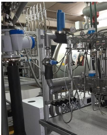
Figure 3: Detailed view of the sampling unit. At the bottom, there are various connected sampling ports from different points of the system, including one fresh-water port. The first cell contains the specific hydraulic conductivity sensor, while the one on top contains the pH and redox sensors. The pipes are insulated to minimize thermal losses.
