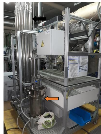
Figure 2c: Back view of the second rack of the hardware twin. The black arrow indicates to the residence time section of both strands and the orange arrow indicates the pressurized reaction vessel.
