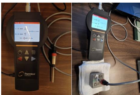
Figure 1: Measurement Platform -2 (MP 2) with 50 mm probe for the measurement of thermal conductivity.
