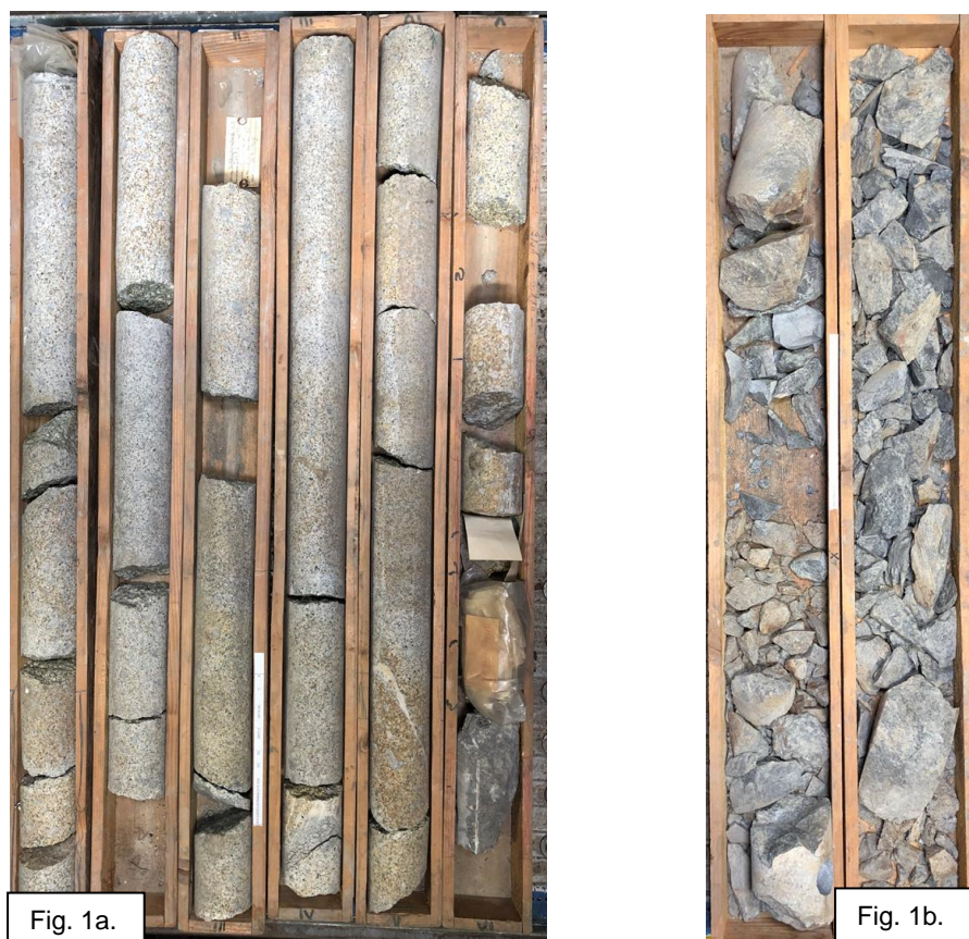
Fig. 1a: Example of good quality core interval. Fig. 1b: example of poor quality core interval.
