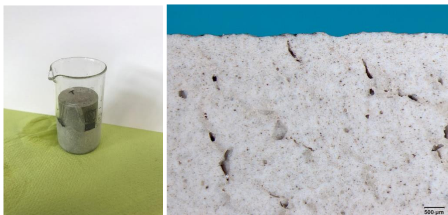
Figure 3: left: cement sample placed in brine from Krummhörn, right: microscopic image of the cement core's boundary area
