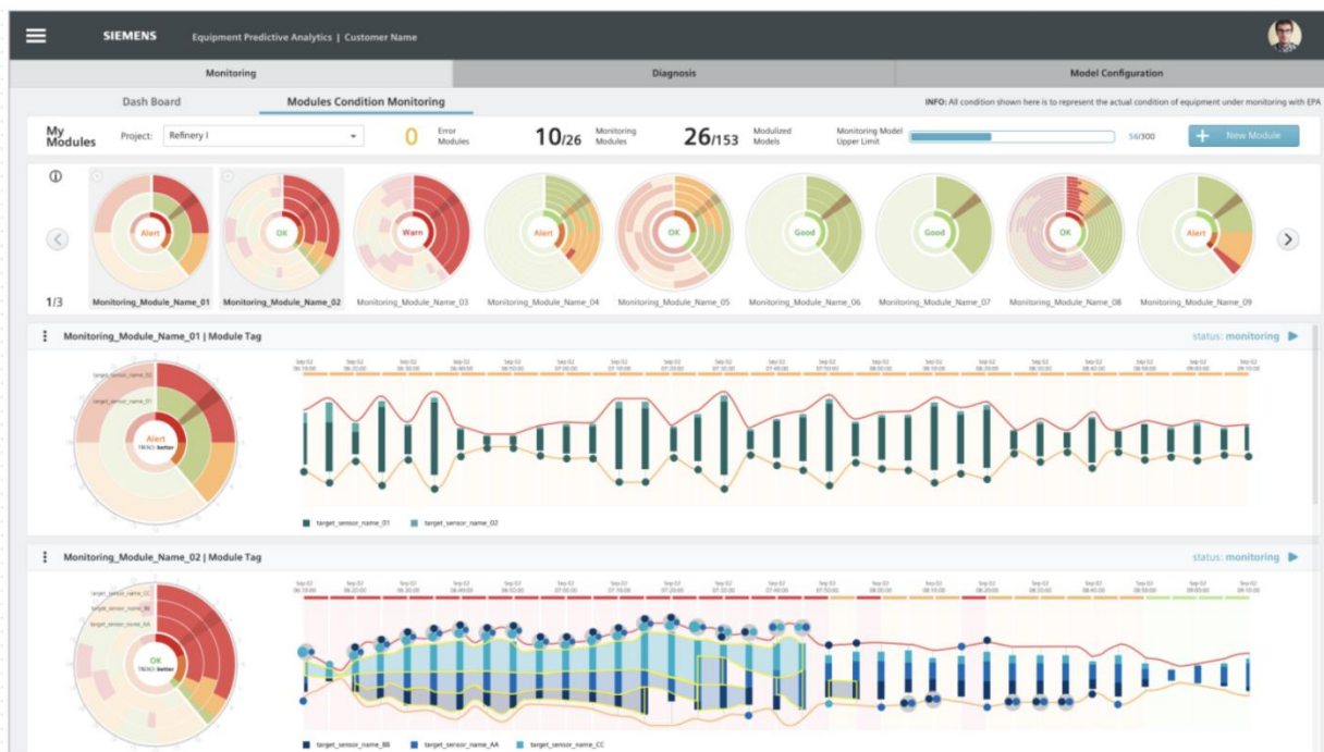
Figure 1 SiePA dashboard with target sensors grouped into modules (sunburst charts), a timeline with the status, and bar charts (as DNA charts) for target sensor deviation.
