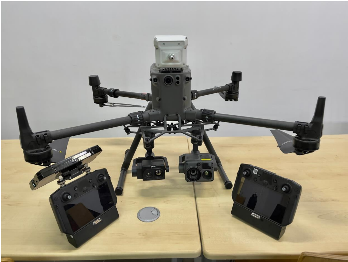
Figure 2: UAV Matrice 300 RTK with controls, cameras and sensors
