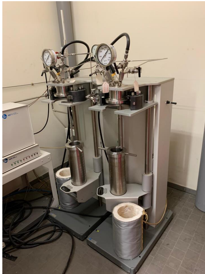
Figure 7: Setup used for cement ageing in presence of CO 2 .
