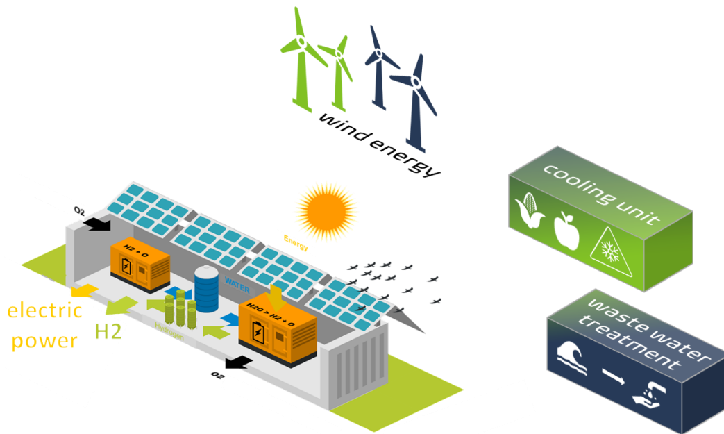
Figure 3: extension options of the microgrid
