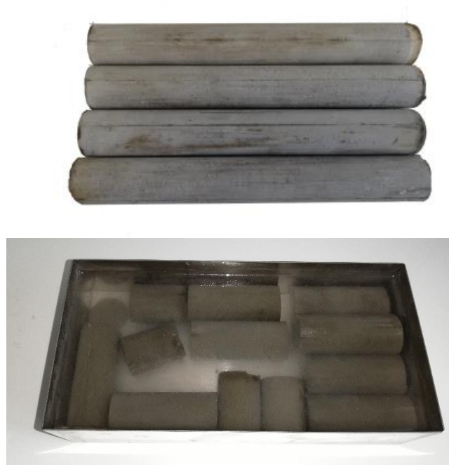
Figure 4: Cement samples before (top) and after cutting (bottom).
