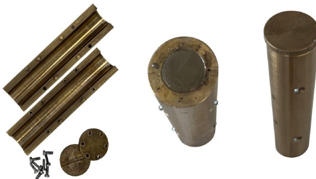
Figure 3: Mold for cement slurry curing: left = disassembled, middle = filled with cement slurry and right = closed with a lid.
