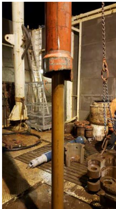
Figure8: Overshot to fishing drilling pipe
