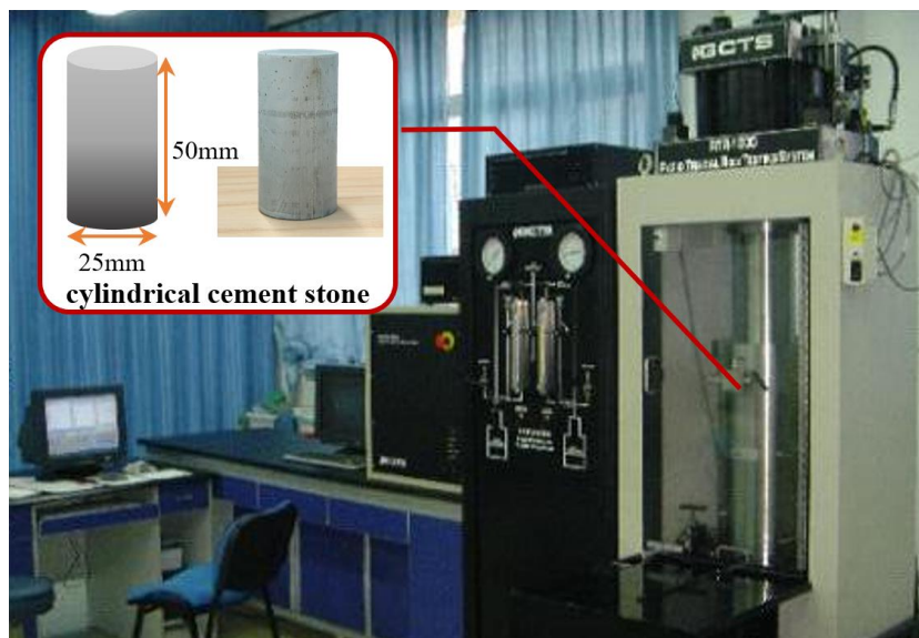
Figure 5. Rapid rock triaxial testing system and cement stone specimen.
