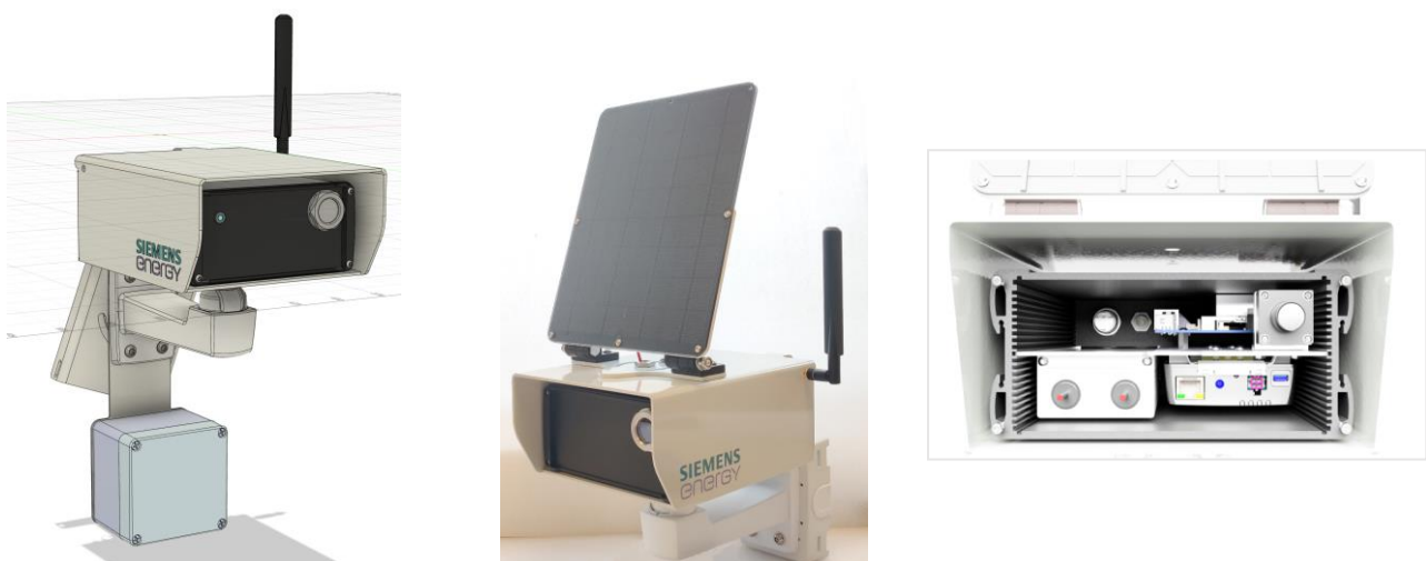
Figure 4 – Second version with custom case; solar powered variant (middle), placement of components inside the case (right)
