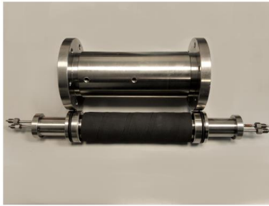
(b) Sleeve sealed with gaskets connected to capillaries ( bottom ) and pressure cell ( top )
