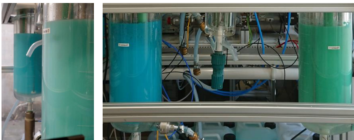
Figure 7. Color change during aging: the reactors in the background and on the left respectively show a blue color before the phase change begins ( t_{\text{age}} \ll t_{\text{change}} ). The reactors in the front and on the right respectively are greenish after zincian malachite was formed ( t_{\text{age}} \gg t_{\text{change}} ).
