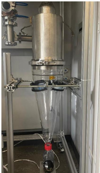
Figure 1. Cyclone for solid separation from the effluent stream.
