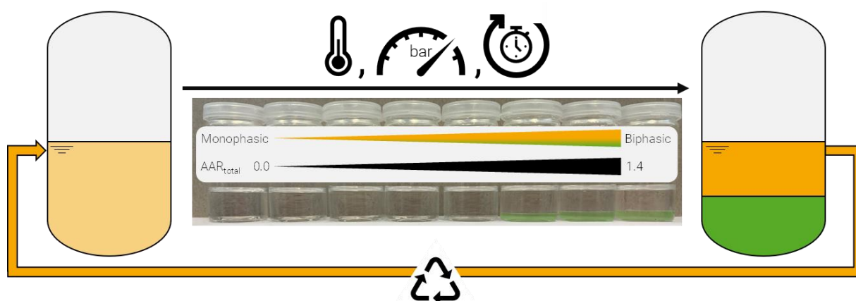
Figure 1 Illustration of the reaction system with self-separating product phase
