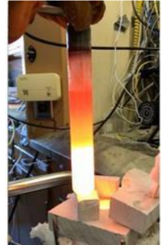
Ni-Bi bubble column reactor
