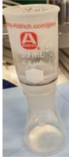
Pore size – 4 – 8 \mu\text{m}
