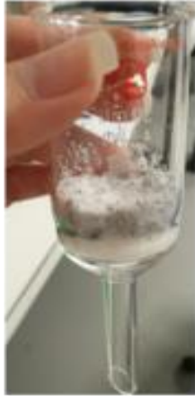
Pore size – 4 – 8 \mu\text{m}
