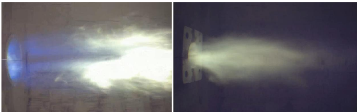
Figure 5: Natural Gas (left) and \text{NH}_3 flames (right) using full scale burners
