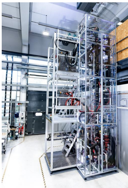
Figure 1: PN50 distillation column with a total height of 7.5 meters at Fraunhofer ISE, serving as a platform for DME and SAF process development.
