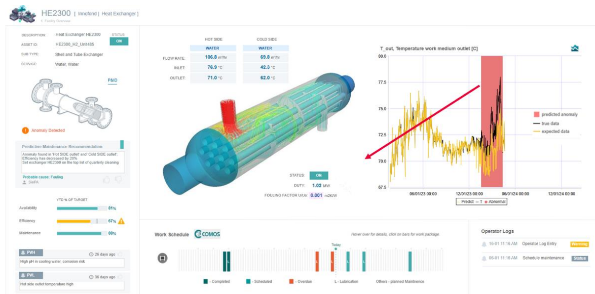
Figure 6 - Predictive Maintenance using Anomaly Detection for a Heat Exchanger
