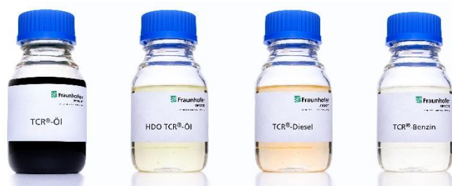
Figure 3: Visual comparison of raw bio-oil, hydrotreated oil and upgraded fuel fractions
