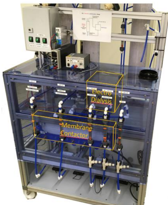
Figure 5: Lab plant used for flue gas treatment experiments
