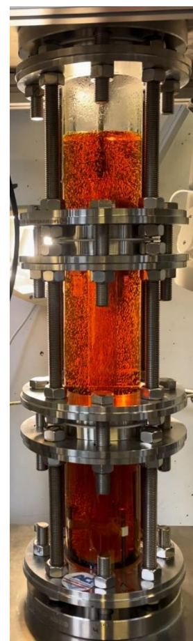
Figure 1: Oxidation of a glycerol solution within the jet loop reactor using a POM catalyst.
