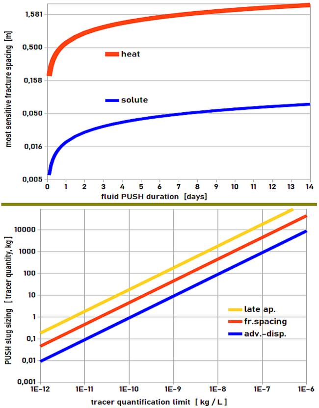
The transport parameter sensitivity of heat or solute tracer 'pull' signals depends on 'push' slug sizing
