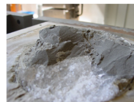
Sheared interface between borehole cement and salt
